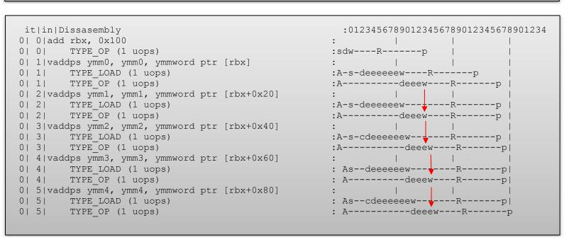
As seen in the trace output, unrolling the loop gives a significant performance gain. The vaddps operations seen in the top trace output are dependent due to ymm0, and so each Operation is performed only after the previous operation reached writeback stage. Unrolling the loop makes use of more registers and so parallel executions are possible.
