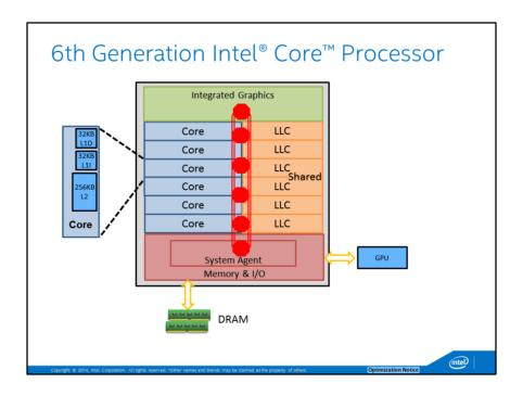
This image represents a general CPU layout and is intended to help illustrate the concepts described in this guide. It is not designed to be a definitive representation of the microarchitecture.
